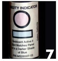
If the humidity indicator card stays pink after one hour or only a partial change has occurred, the test should be repeated with spacer obtained from the reel when 2 layers of the spacer have been unwound. If the result is still not satisfactory, please contact your Edgetech Technical representative.
