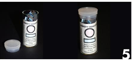
Fill the vial to the top with spacer pieces, and place the cap on securely. Important: Use only FRESH spacer pieces and place in vial IMMEDIATELY.
