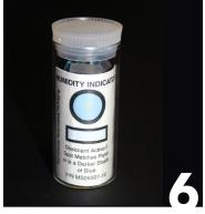
If the Humidity Indicator Card changes to the blue color as indicated on the card, the spacer is deemed acceptable. (Average test time is one hour).
