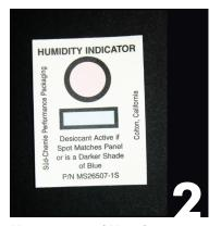
Use an approved Humidity Indicator Card available from Edgetech I.G. Inc. Expose the card to ambient air until round spot turns pink. (Note: Humidity Indicator Cards are reusable).
